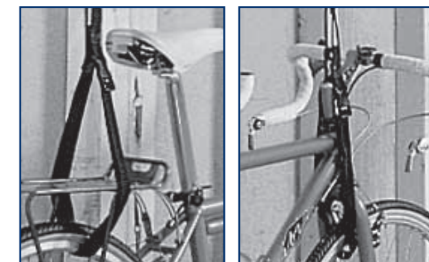
DIAGRAM 21. Locked (left): Single Black/Red Hoisting Rope (F) pointed straight down locks cleat. Open (right): Angled rope opens cleat.
